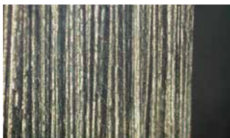
con lima racing / with racing file - Ra=0.90
